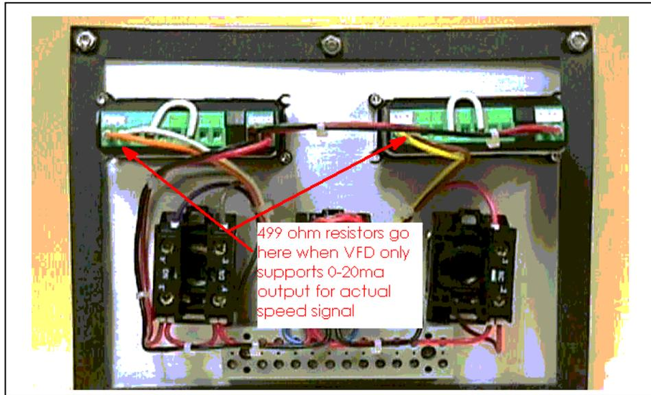
**Figure 5 - Current Loop Resistor Installation Points**
